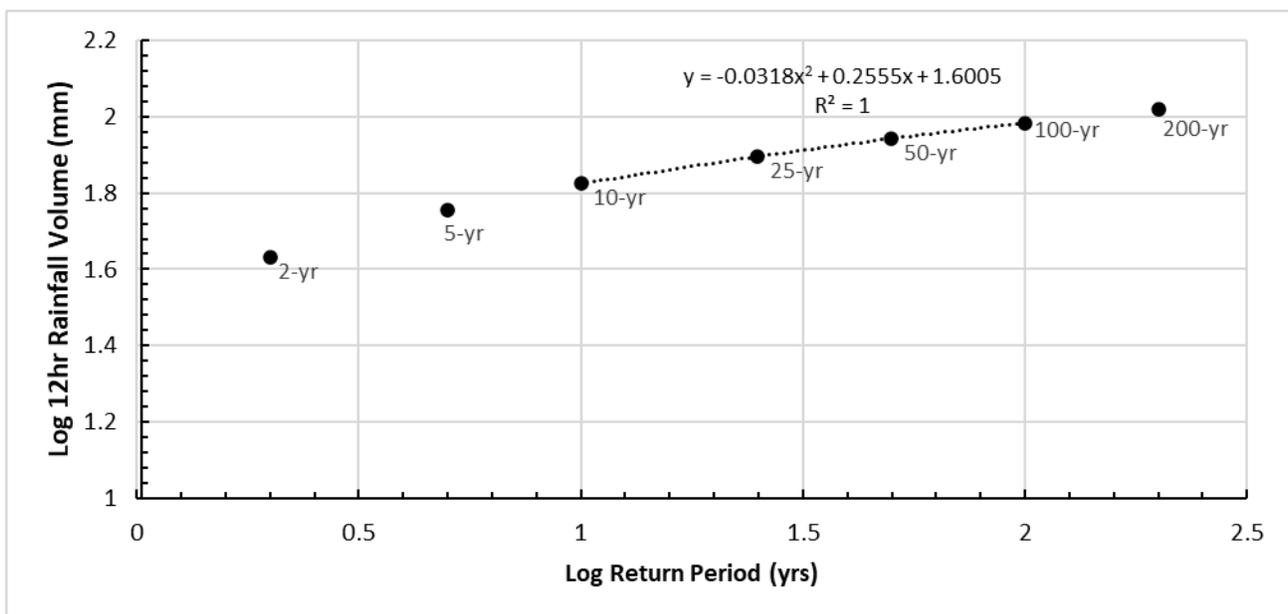
**Figure 4-5. Log-Log Plot of 12-hr Storm Rainfall Depths vs. Return Period with Line of Best Fit**
