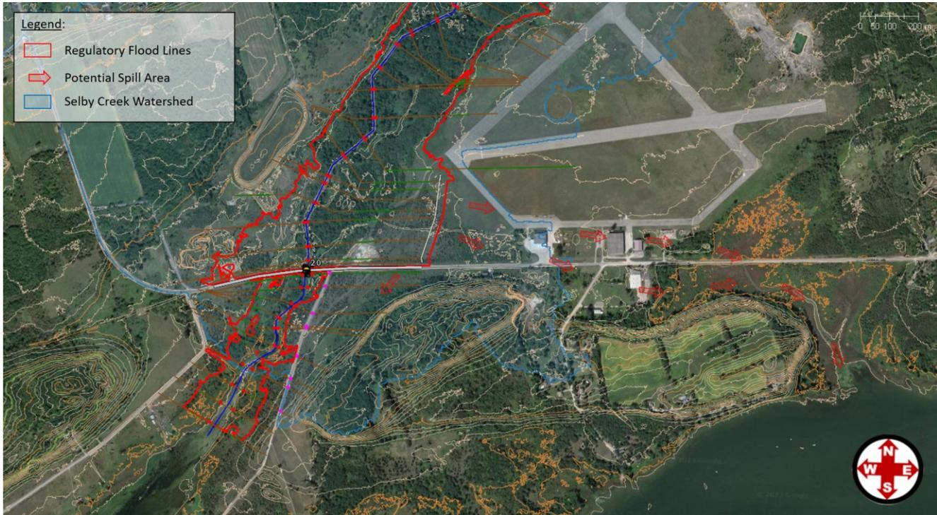
Figure 7-5. Potential Downstream Spill Area in 1D Modelling
