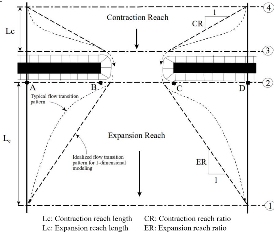
**Figure 7-1. Cross-Section Locations at Crossing Structures (US Army Corps of Engineers, 2022)**
