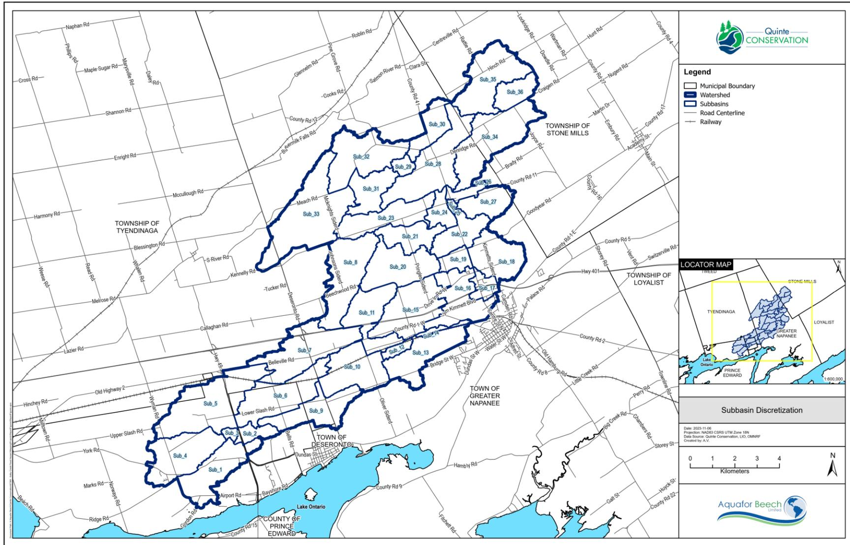
Figure 4-2: Delineated Subbasins in the HEC-HMS Model
