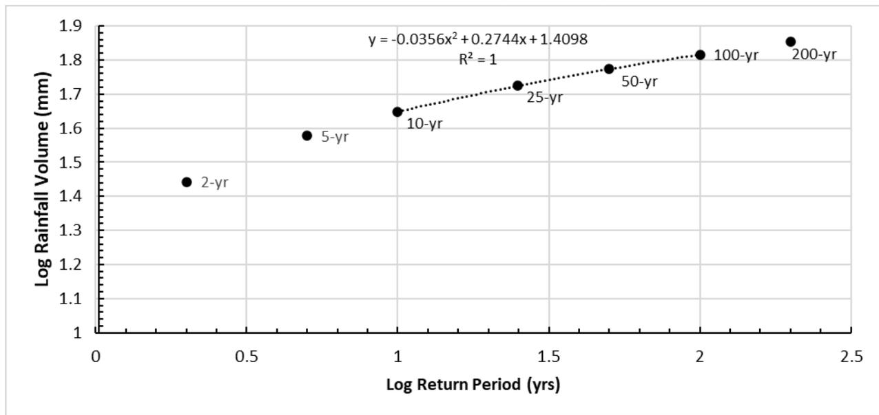
**Figure 4-7. Log-Log Plot of 1-Day Rain-on-Snowmelt Precipitation Depths vs. Return Period, with the Fitted Polynomial Distribution**
