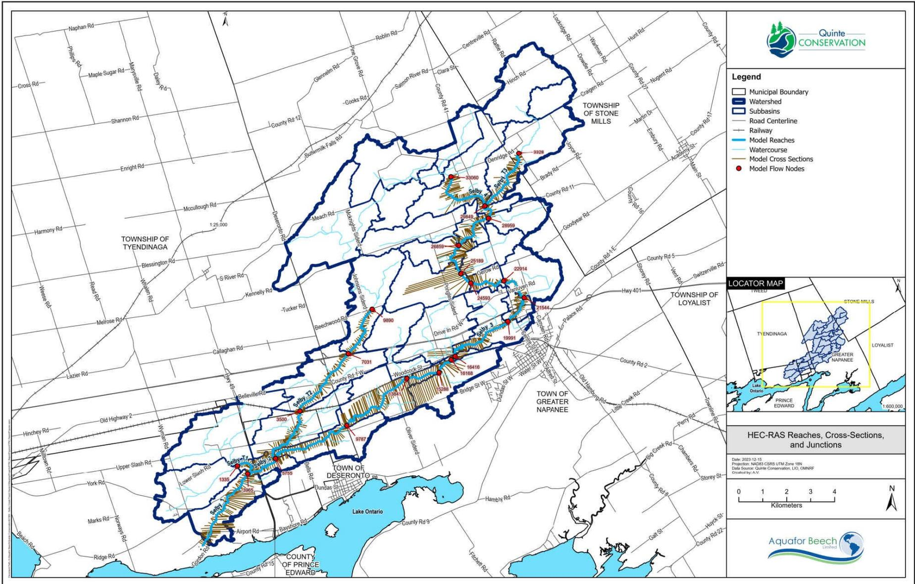
Figure 7-3. HEC-RAS Model Setup and Flow Node Locations
