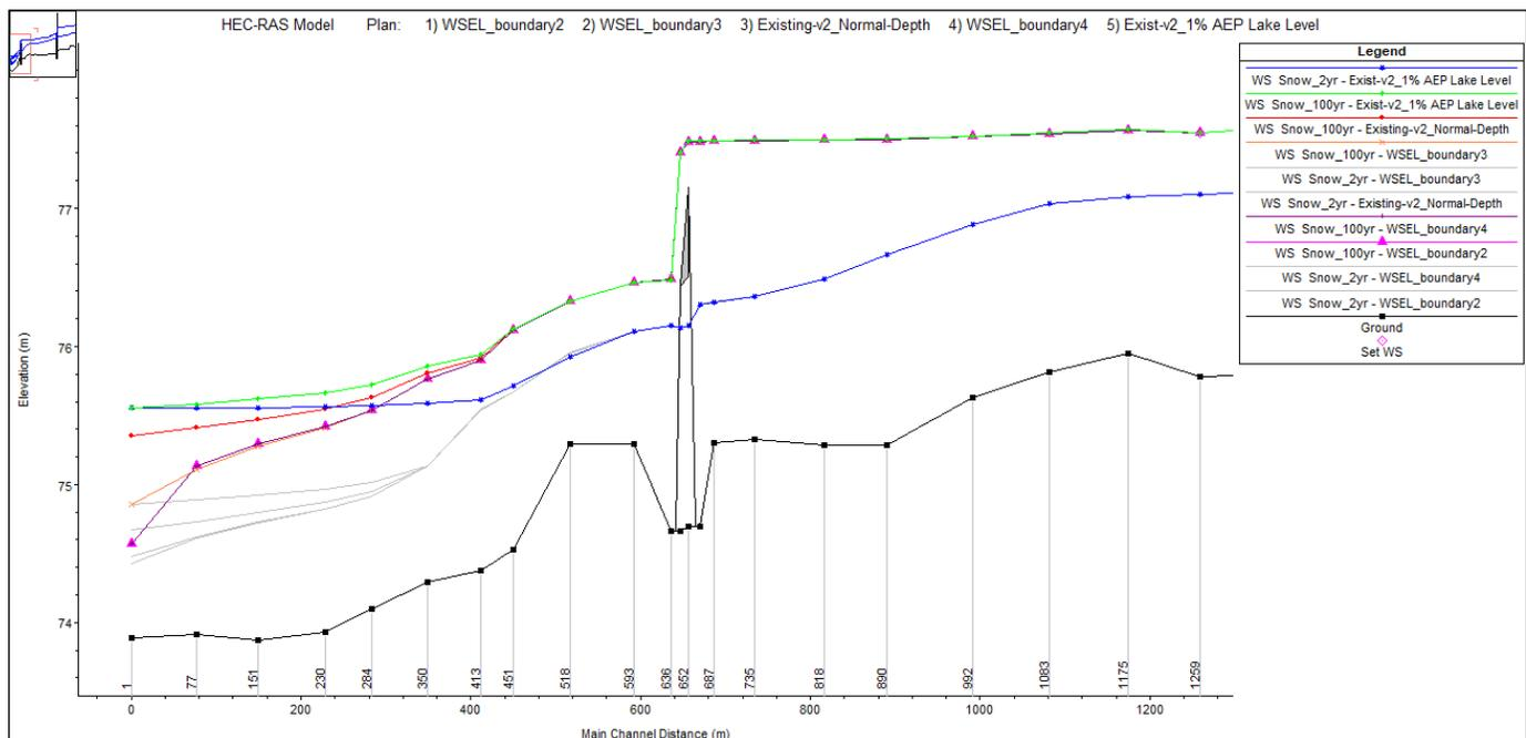
Figure 7-4. Profile Plot Result for the Six Simulated Boundary Conditions Scenarios
