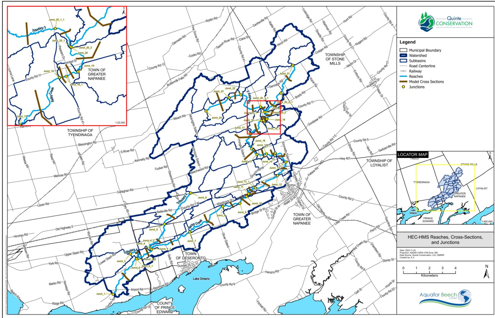
Figure 4-4: HEC-HMS Reaches, Cross-Sections, and Junctions
