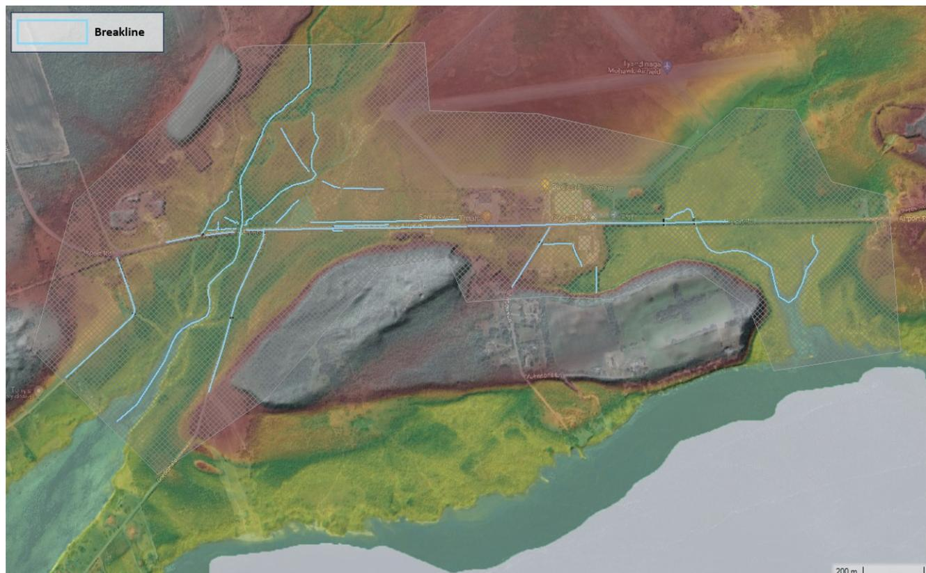
**Figure 8-2. 2D Model Breaklines**
