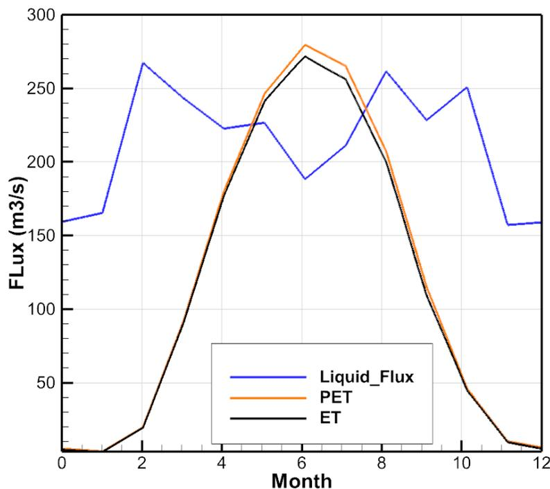
Figure 17. Climatological monthly normal forcing data for the HGS model spinup, along with simulated evapotranspiration rates for a one-year climate cycle.
