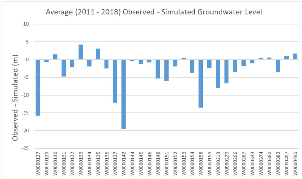
Figure 26. Difference in long term (2011 – 2018) daily average observed and simulated groundwater levels in the 31 PGMN wells used to evaluate model performance.
