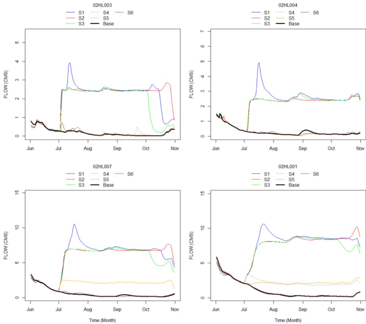
Figure 30. Simulated flow rates at hydrometric stations located along the **Moira River**, during the June to November 2016 time interval, for the **first set of reservoir evaluation scenarios**.
