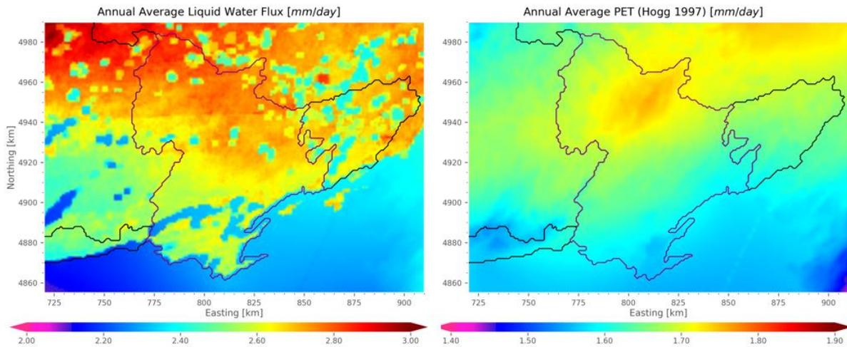
Figure 19. (Left panel) 2011 to 2018 average spatial distribution of liquid water flux (LWF) over the model domain. (Right panel) 2011 – 2018 average spatial distribution of potential evapotranspiration (PET) over the model domain.
