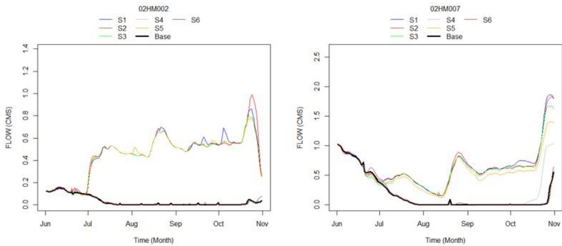
Figure 32. Simulated flow rates at hydrometric stations located along the **Napanee River**, during the June to November 2016 time interval, for the **first set of reservoir evaluation scenarios**.
