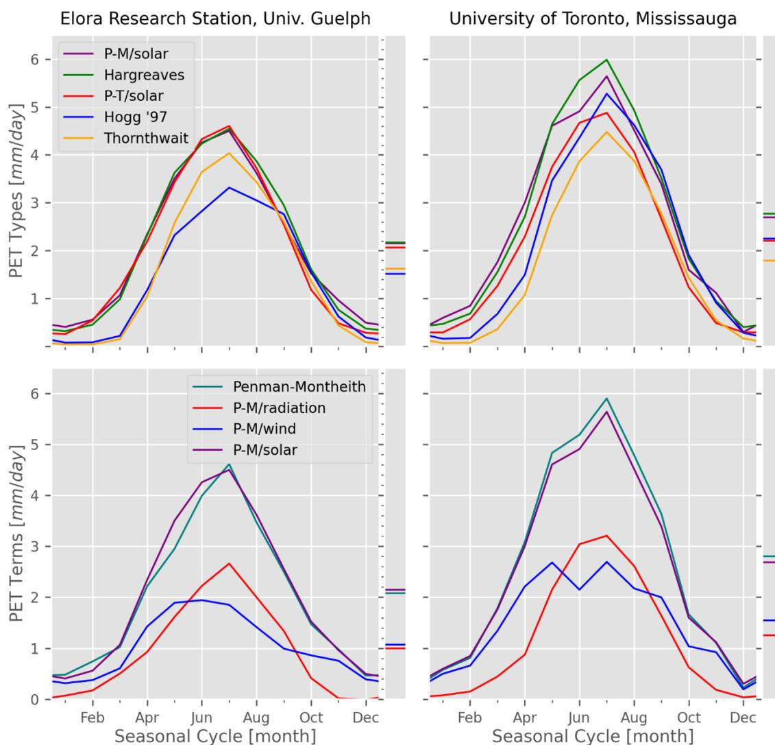
Figure 20. (top row) Comparison of different PET estimation methods at the Elora (left) and UTM (right) stations; (bottom row) the radiation and wind/aerodynamic terms of Penman-Monteith PET, as well as a comparison of P-M calculated with just solar radiation (estimated LW radiation; 'solar') vs. full net radiation; P-M and P-T in the top row only use solar radiation (estimated LW). The vertical bars on the right-hand side of each panel show the annual average of each variable.
