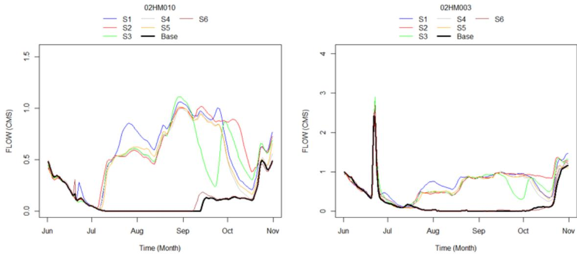
Figure 31. Simulated flow rates at hydrometric stations located along the **Salmon River**, during the June to November 2016 time interval, for the **first set of reservoir evaluation scenarios**.
