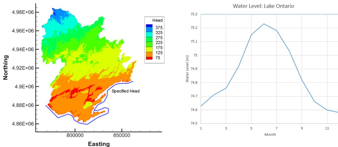
Figure 16. Time-varying head boundary condition configured into the Quinte HGS model to reflect seasonally varying water levels in Lake Ontario.
