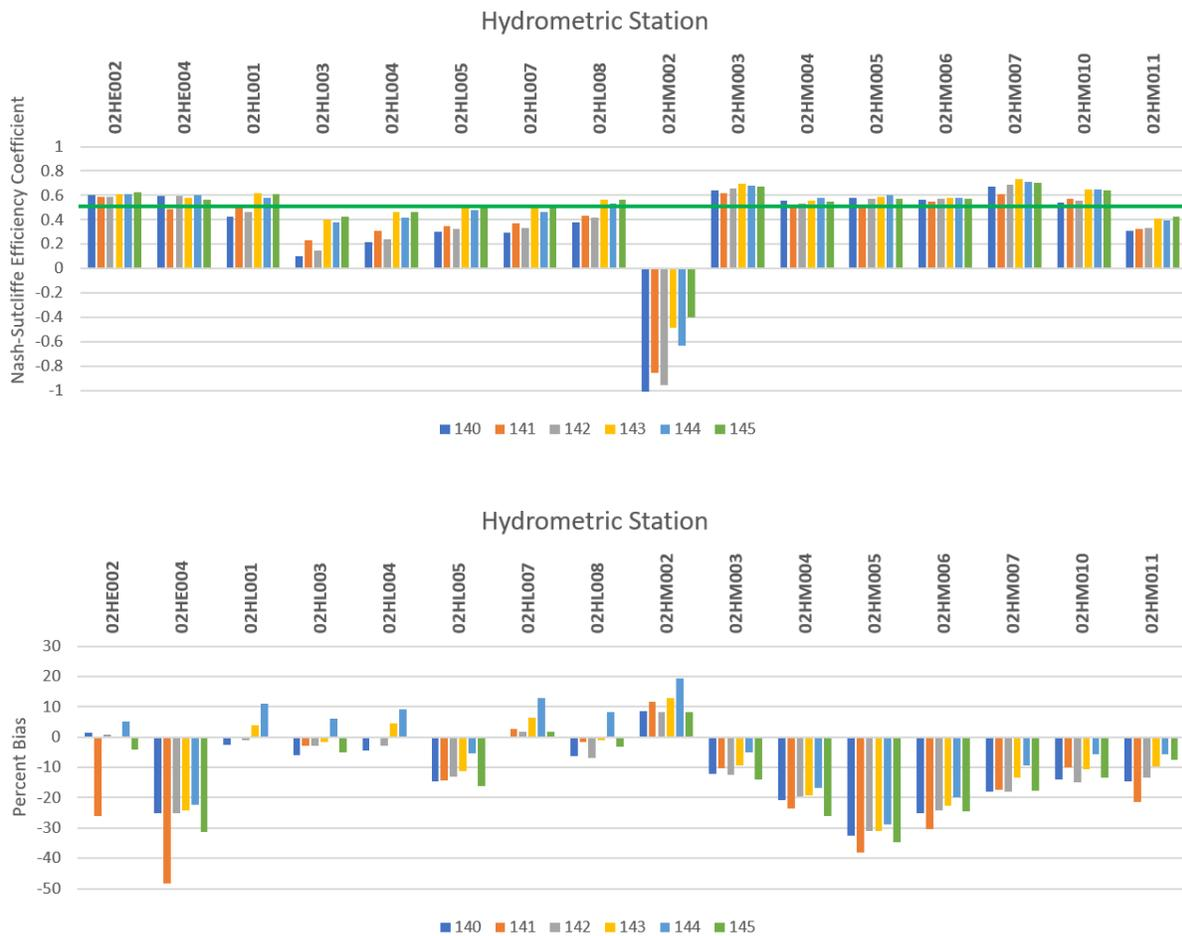
Figure 23. Nash-Sutcliffe model efficiency (NSE) coefficient (top frame) and Percent Bias (bottom frame) for the six different model configurations tested during the performance evaluation. Performance metrics represent daily comparison of simulated versus observed flow rates at sixteen hydrometric gauging stations.
