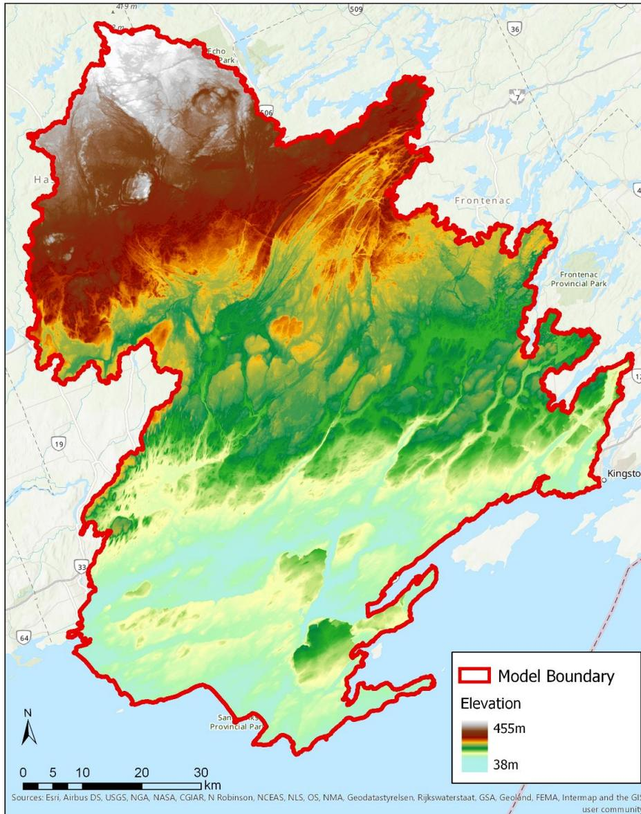
Figure 4: Stitched Ontario Integrated Hydrology DEM, NOAA bathymetry, and inland lake bathymetry from Quinte Conservation. Resolution 30m in UTM 17N.
