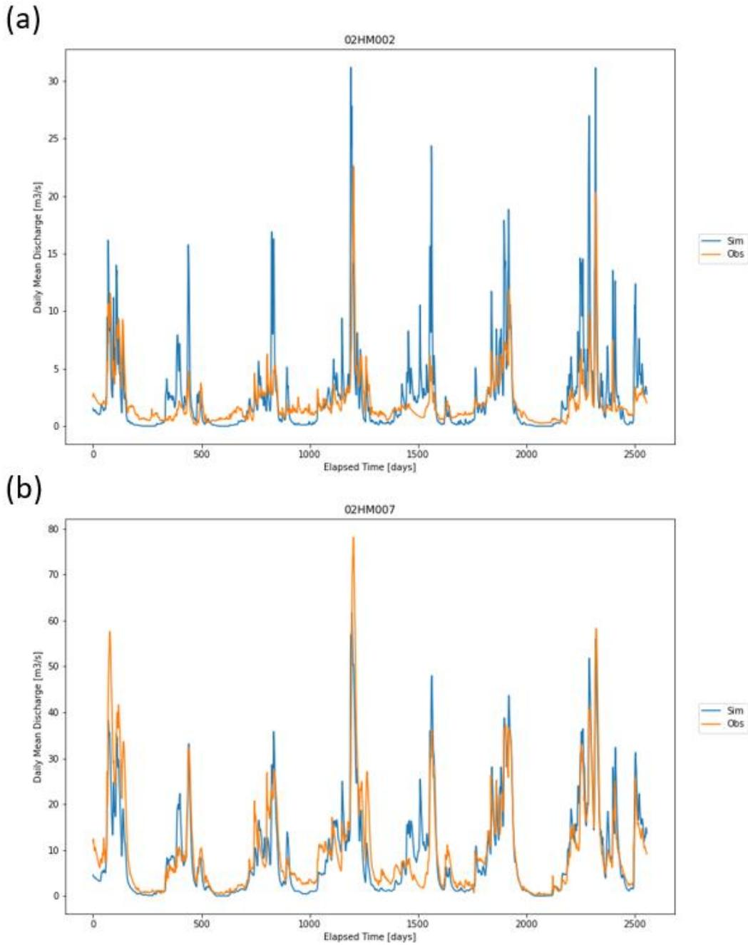
Figure 24. Simulated versus observed surface water flow rates at the hydrometric station with the (a) lowest, and (b) the highest NSE values. Note that Day 0 represents January 1, 2011 and the time series extends to Day 2555, which reflects December 31, 2018.
