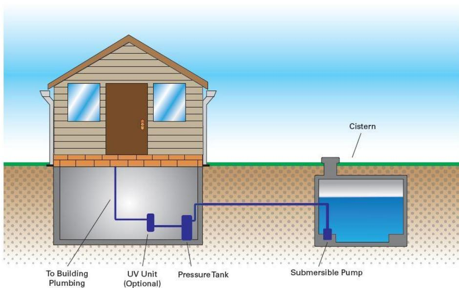
To prevent water from freezing, cisterns are usually buried below the frost line or located inside of a heated building such as the basement of a home. Cisterns must have an access point, a water tight lid, a fill point and a vented overflow pipe. Cisterns need to be sized according to anticipated demand and keeping in mind that the longer water is stored the greater the risk of stagnant water and potential microbiological contamination.
