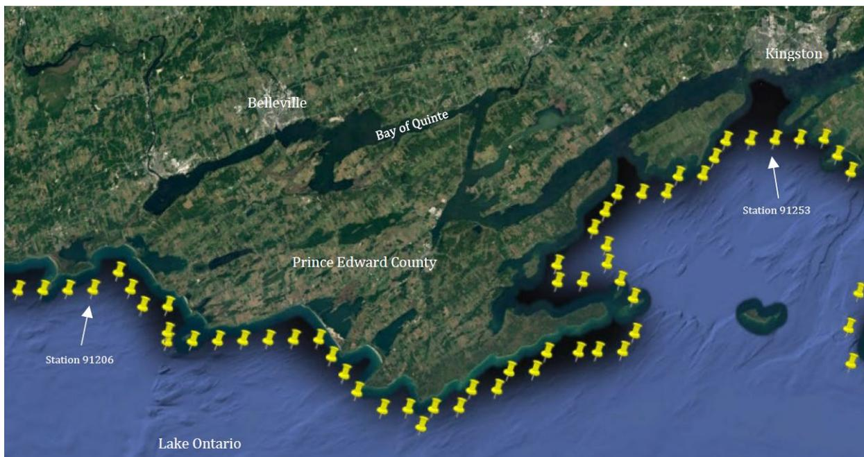
**Figure 4.22 Wave output locations from the WIS study located within the project geography (USACE)**
