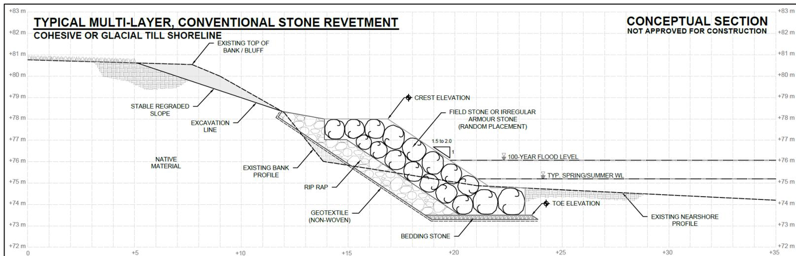
Figure 7.18 Typical multi-layer, randomly placed stone revetment for a cohesive or glacial till shoreline (concept only)
