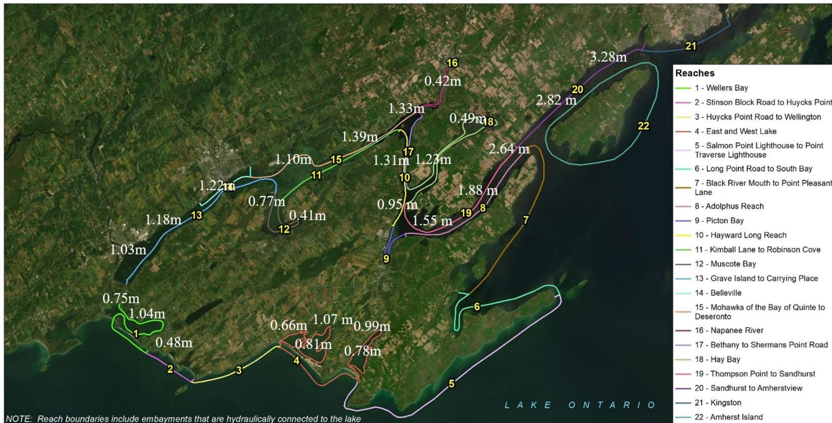
Figure 4.30 Estimated 100-year significant wave height (meters) throughout the Bay of Quinte and other sheltered embayments
