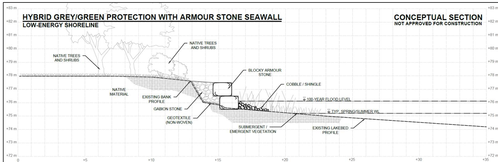
**Figure 7.23 Aspects of a hybrid grey-green shoreline protection scheme for sheltered embayments and other low wave energy environments featuring a stacked armour stone seawall (concept only)**
