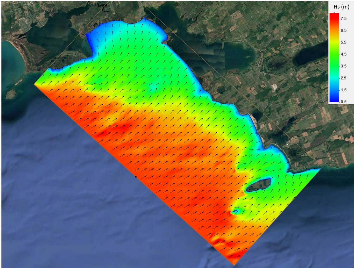
**Figure 4.26 Modelled significant wave height (colour contours) and direction of wave propagation (vectors) for the 25-year event from Wellers Bay to Huyck’s Point (Model A)**
