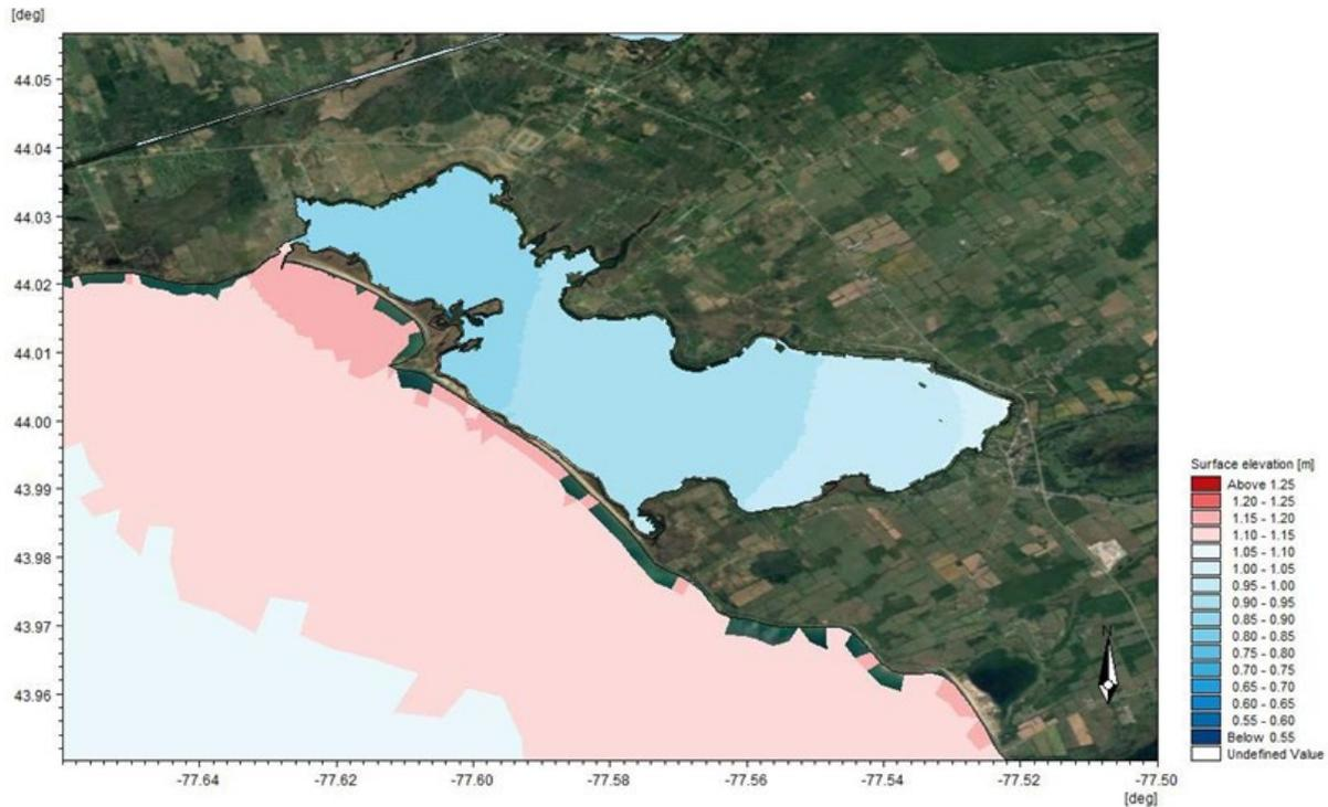
**Figure 4.16 Simulated storm surge gradient within Wellers Bay during the April 6, 1979, storm event (in metres above Chart Datum)**
