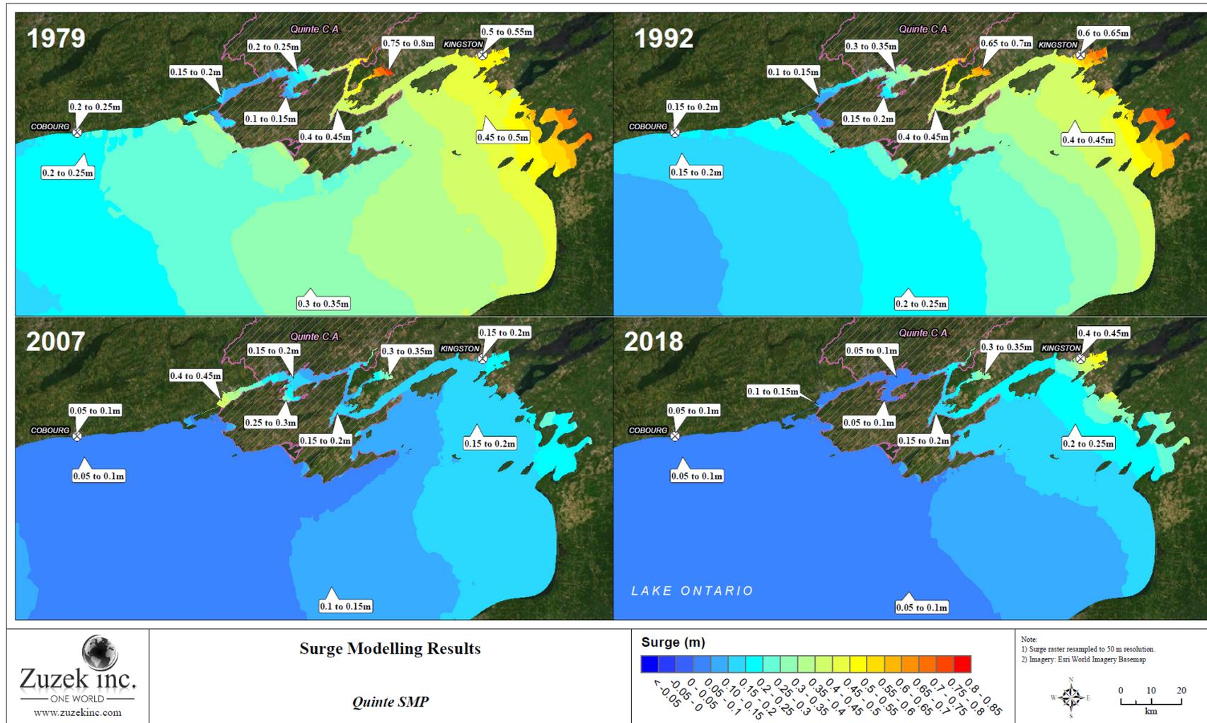
Figure 4.19 Maximum surge magnitude (in metres) experienced throughout the model domain during the four (4) simulated surge events
