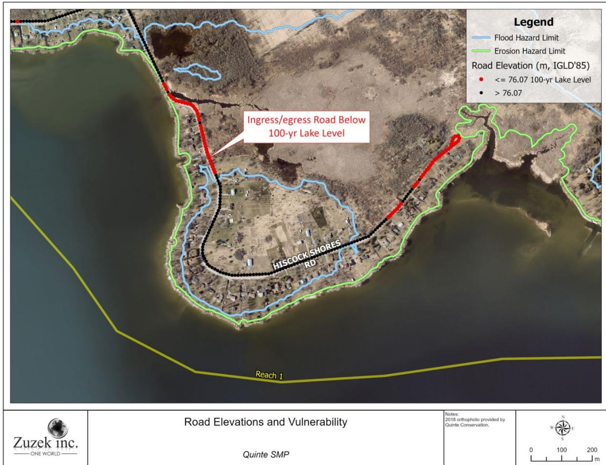
**Figure 5.4 Example of a community without safe ingress/egress (emergency access) during the 100-year flooding event, at Hiscock Shores Road, Wellers Bay (Reach 1)**
