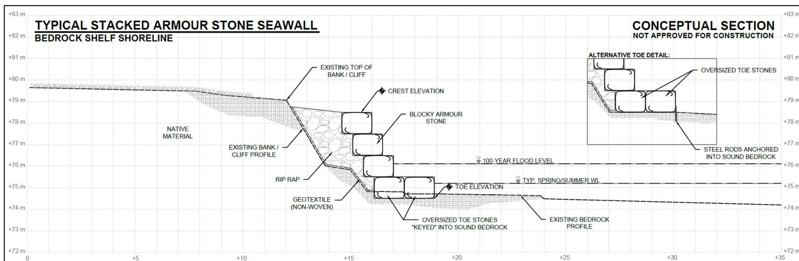
Figure 7.20 Typical stacked armour stone seawall founded on a bedrock shelf (concept only)
