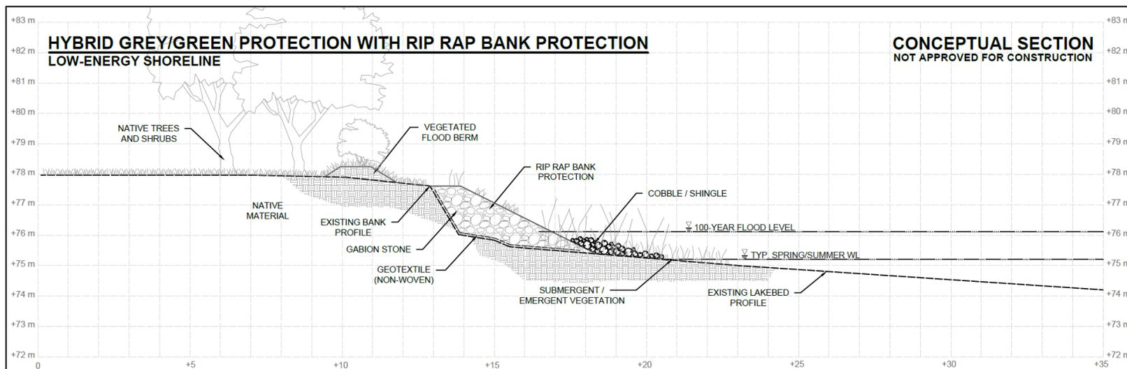
Figure 7.22 Aspects of a hybrid grey-green shoreline protection scheme for sheltered embayments and other low wave energy environments featuring a vegetated rip rap slope (concept only)
