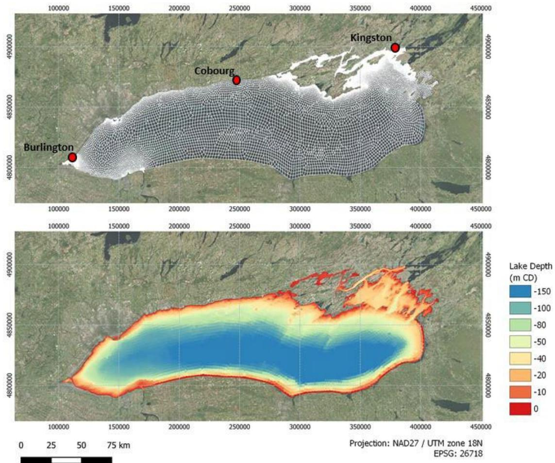
**Figure 4.11 Lake Ontario surge model mesh (top) and interpolated bathymetry (bottom)**
