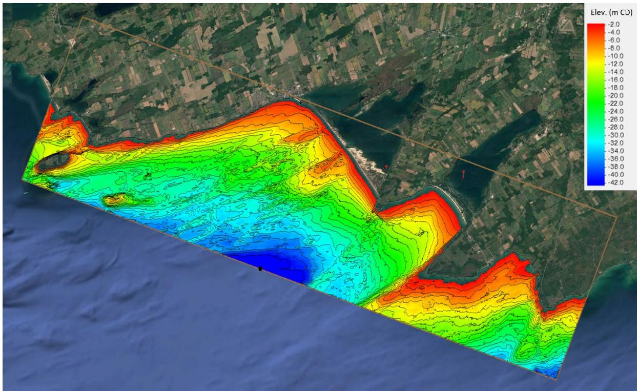
**Figure 4.25 Nearshore wave model (CMS-Wave) domain and bathymetric contours for Model B, from Huyck's Point to Point Petre**
