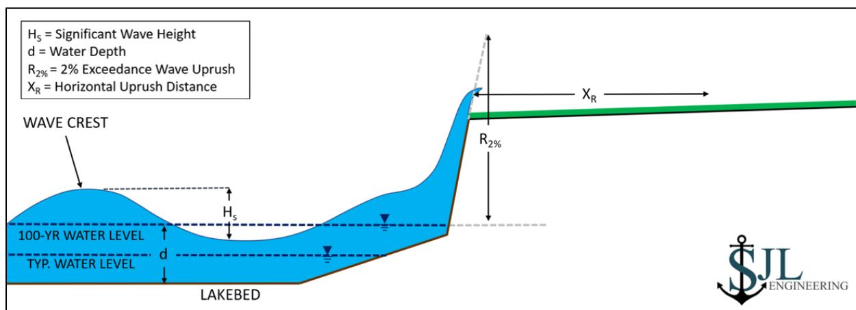
**Figure 4.34 Wave uprush on a steep bank or cliff resulting in overtopping of the bank crest**
