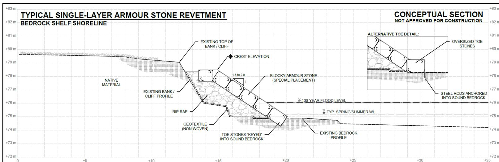
Figure 7.19 Typical single-layer armour stone revetment founded on a bedrock shelf (concept only)
