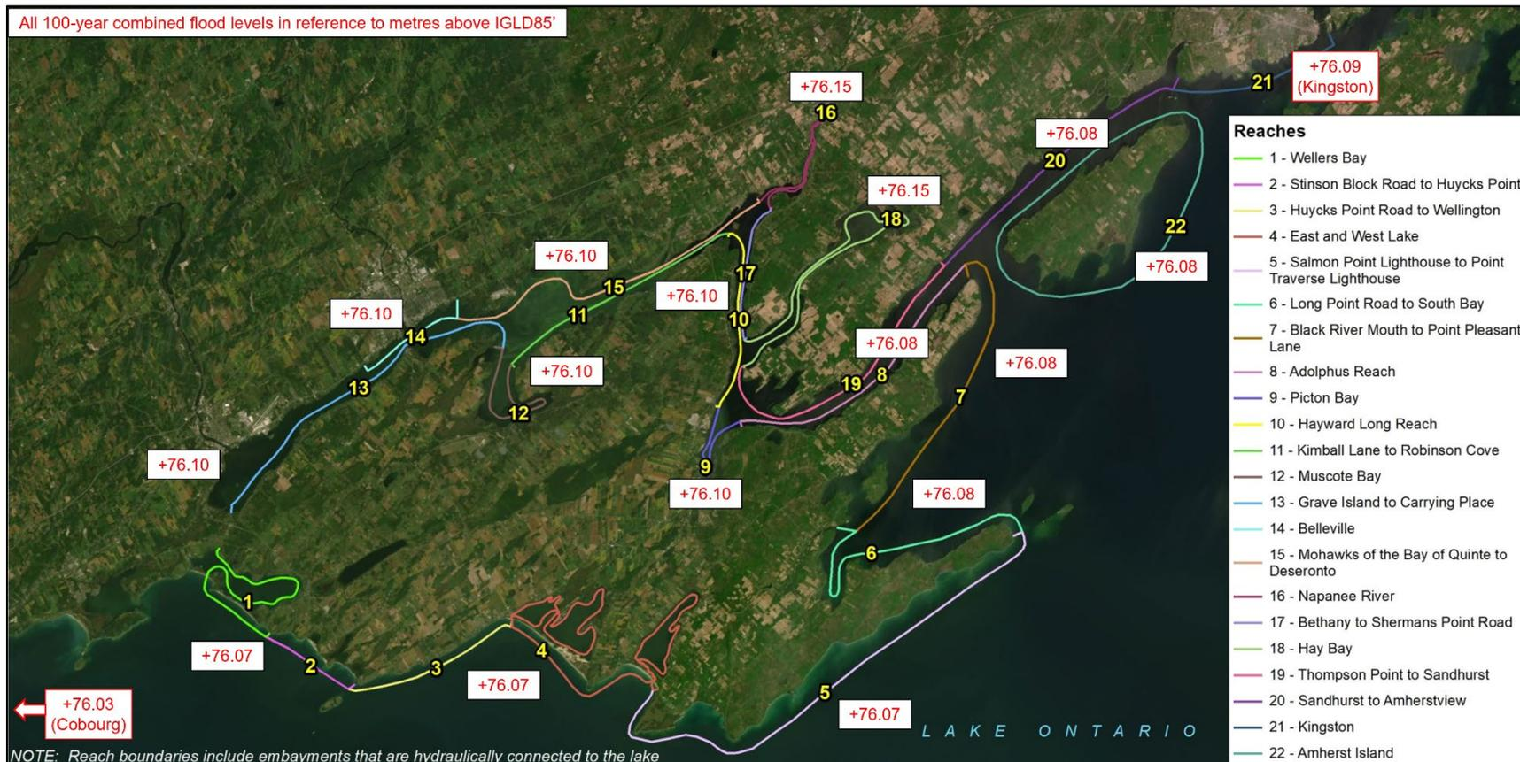
**Figure 4.21 100-year flood levels for entire project geography based on updated joint probability analyses of measured static lake levels (1900 – 2021) and storm surge (1962 – 2021) at Cobourg and Kingston, scaled to other locations using DHI’s high-resolution storm surge model**
