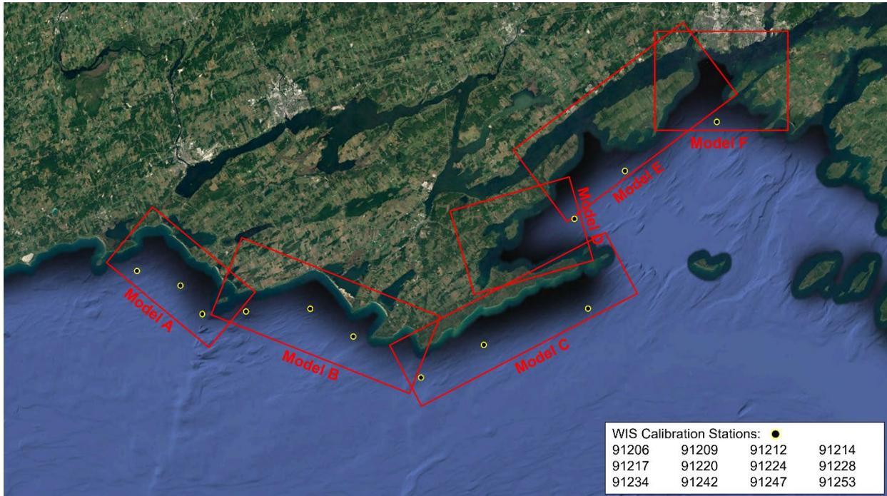
**Figure 4.24 Location, size, and orientation of each of the six (6) numerical wave models used to transform 25-year and 100-year offshore waves to the project shoreline**
