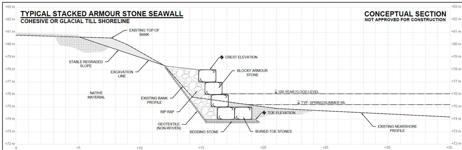
Figure 7.21 Typical stacked armour stone seawall for a cohesive or glacial till shoreline (concept only)
