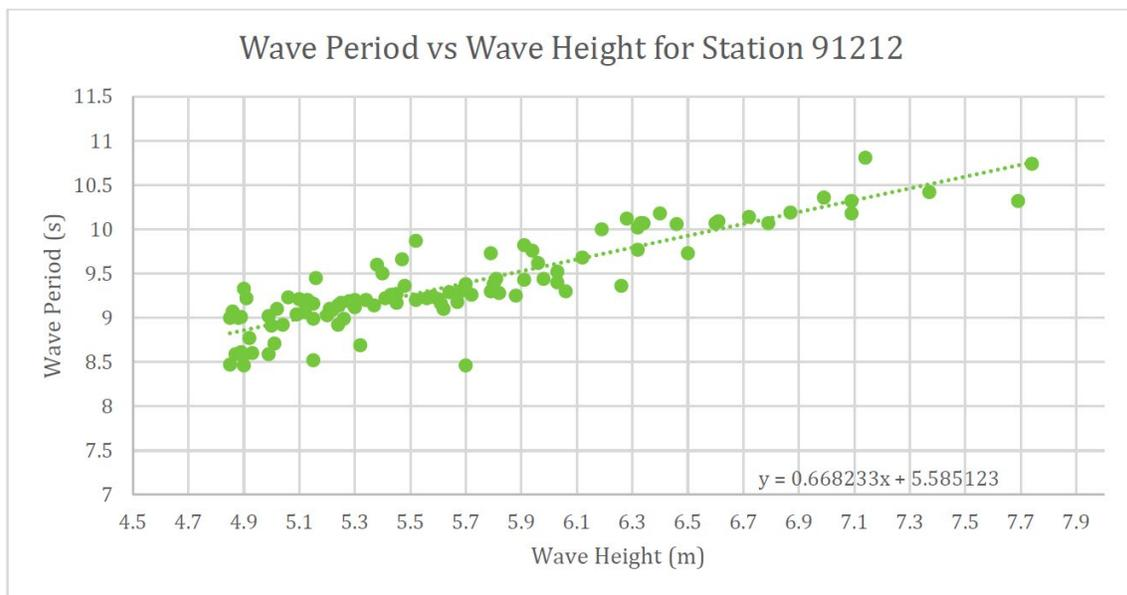
**Figure 4.23 Relationship between significant wave height (Hs) and wave period (Tp) for top 100 storm events at WIS Station 91212**
