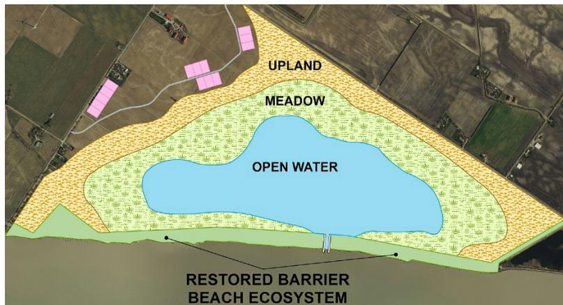
**Figure 7.4 Diked agricultural land located below the lake level converted to a coastal wetland with a restored barrier beach**
