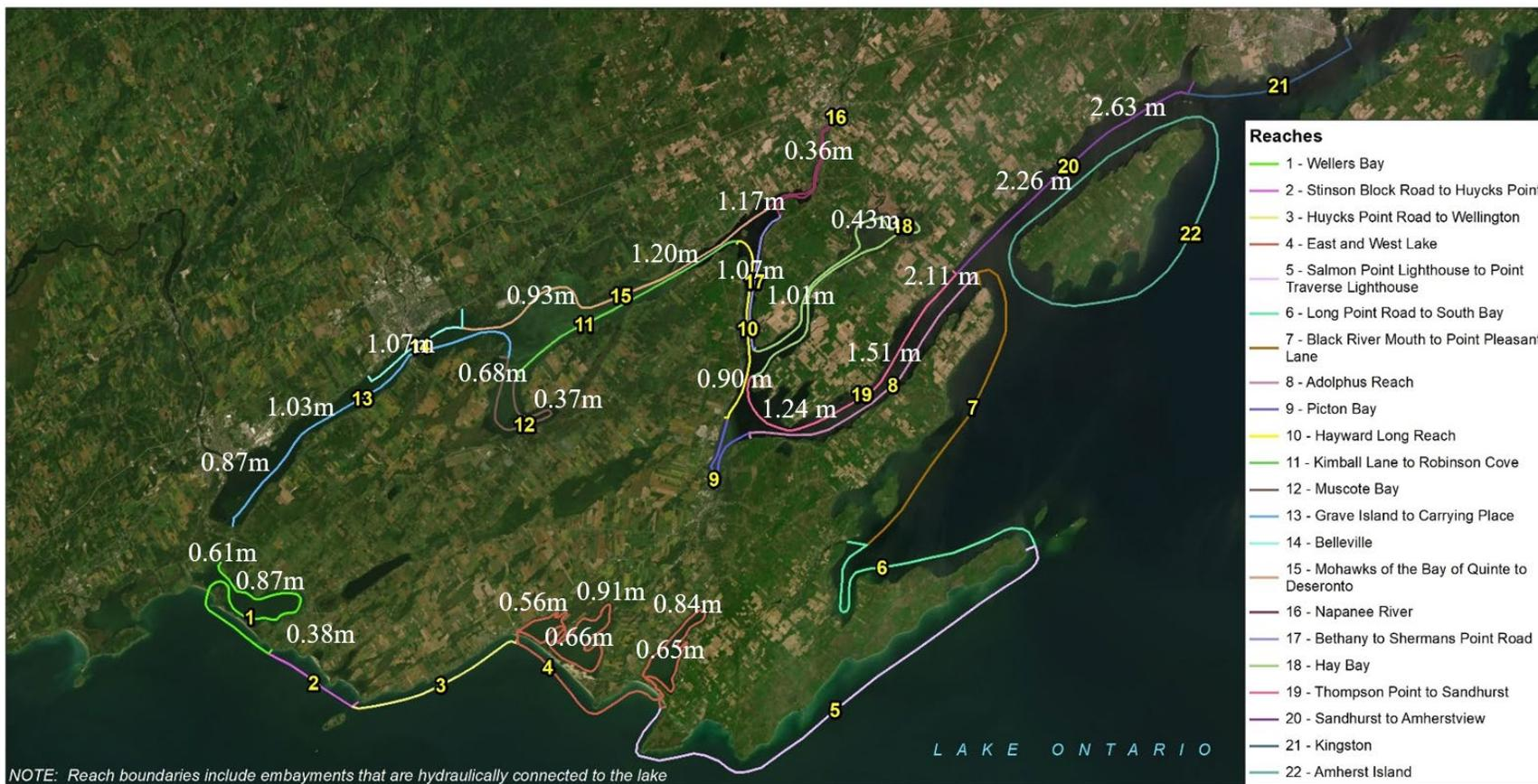
**Figure 4.28 Estimated 25-year significant wave height (meters) throughout the Bay of Quinte and other sheltered embayments**
