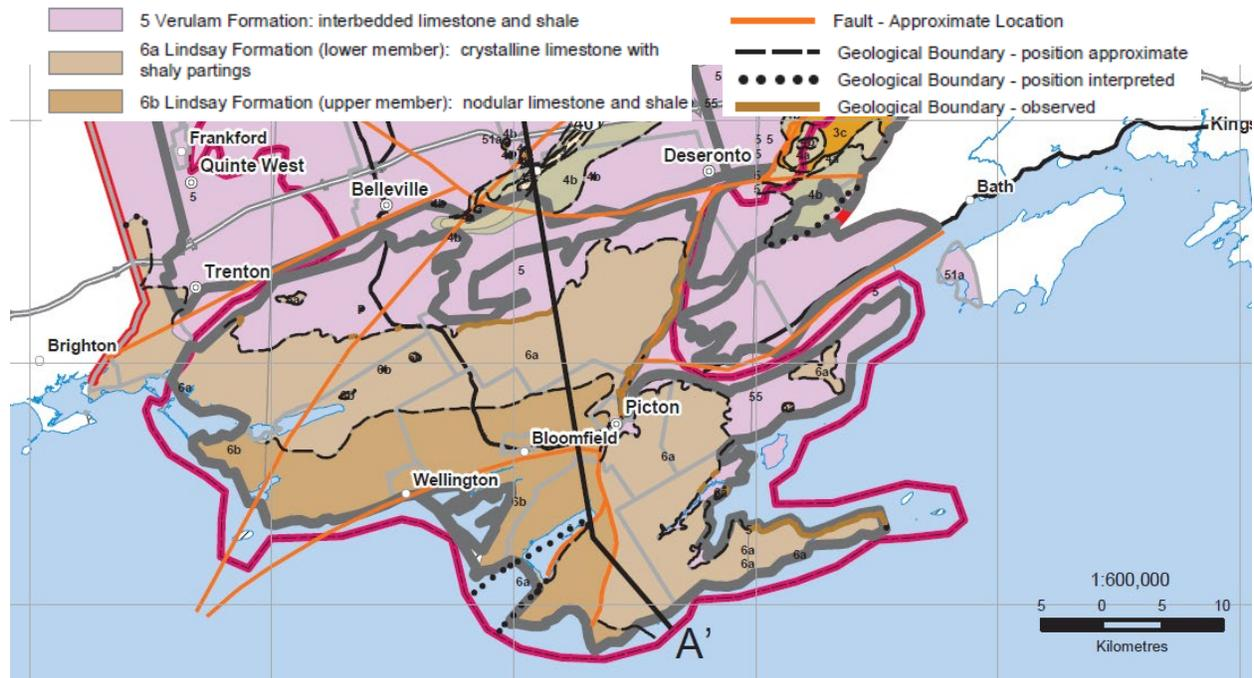
Figure 3.6 Bedrock geology of study area (source: Dillon)
