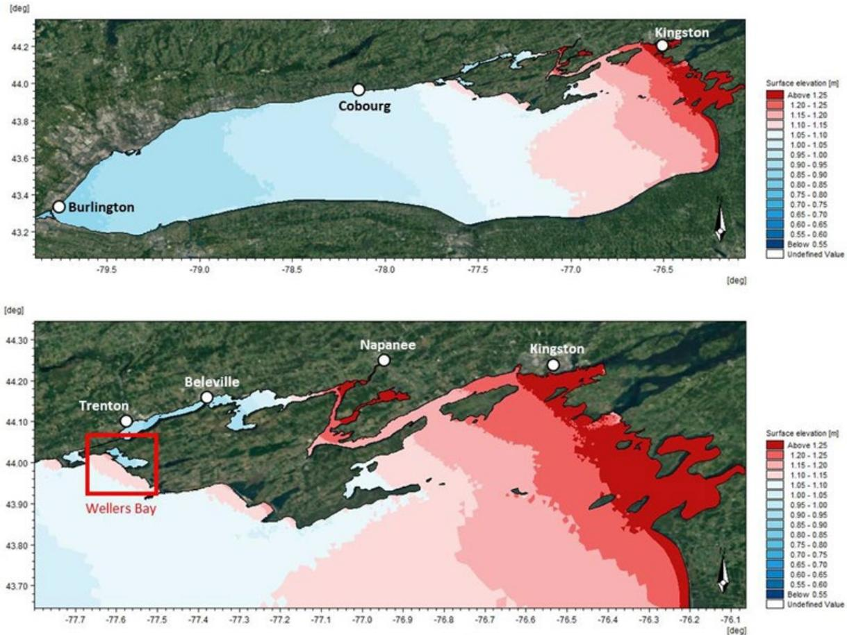
**Figure 4.15 Model output showing maximum water levels across Lake Ontario (top) and the project region (bottom) during the April 6, 1979 storm surge event (in metres above Chart Datum)**
