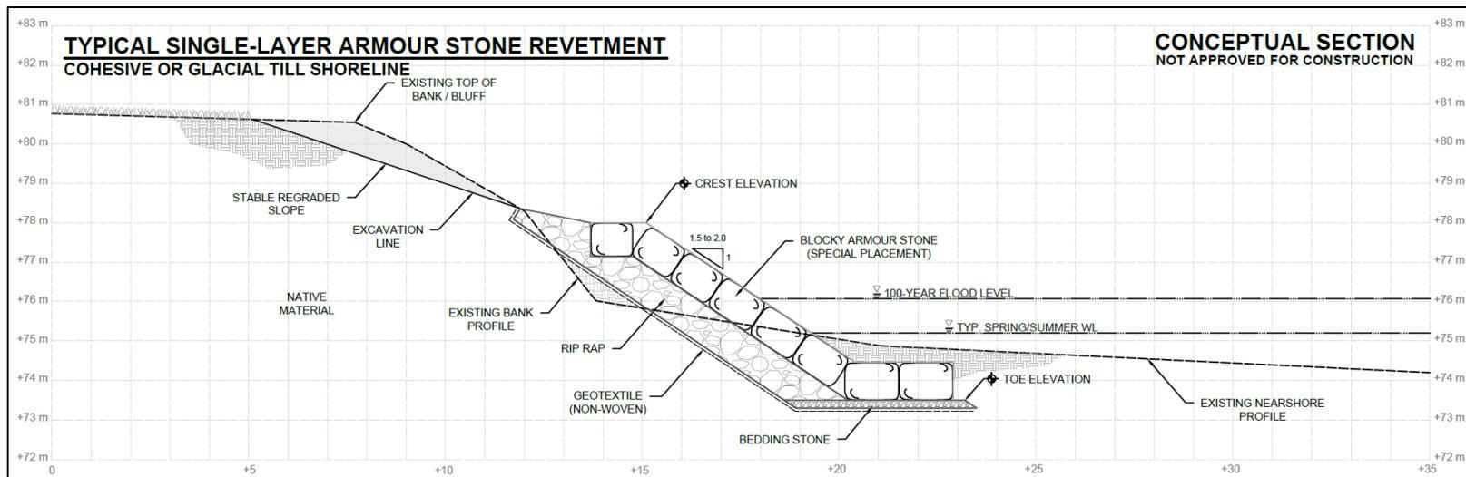
Figure 7.17 Typical single-layer armour stone revetment for a cohesive or glacial till shoreline (concept only)
