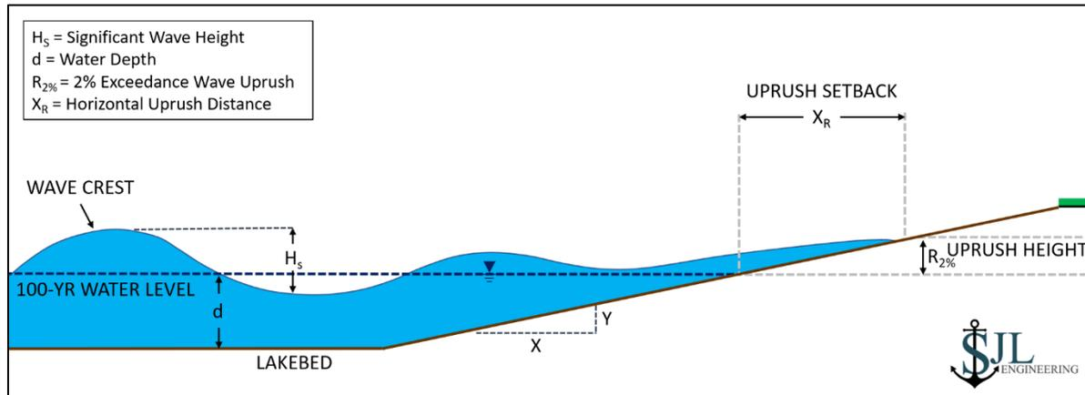
Figure 4.32 Wave uprush on a gentle sloping shoreline – definition sketch
