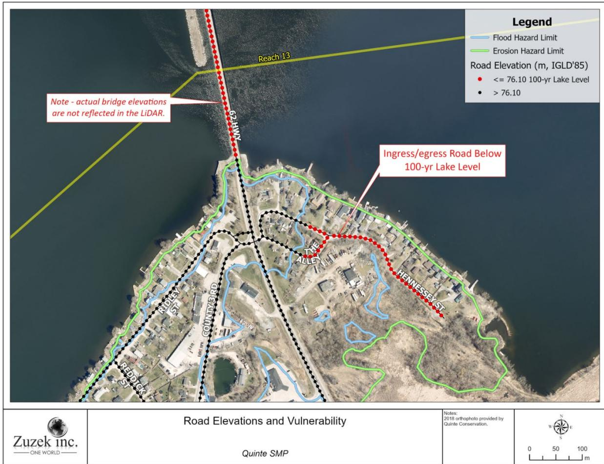
**Figure 5.5 Example of a community where multiple homes are well within the flooding hazard and may be subjected to flood damage and access issues during major flooding events**
