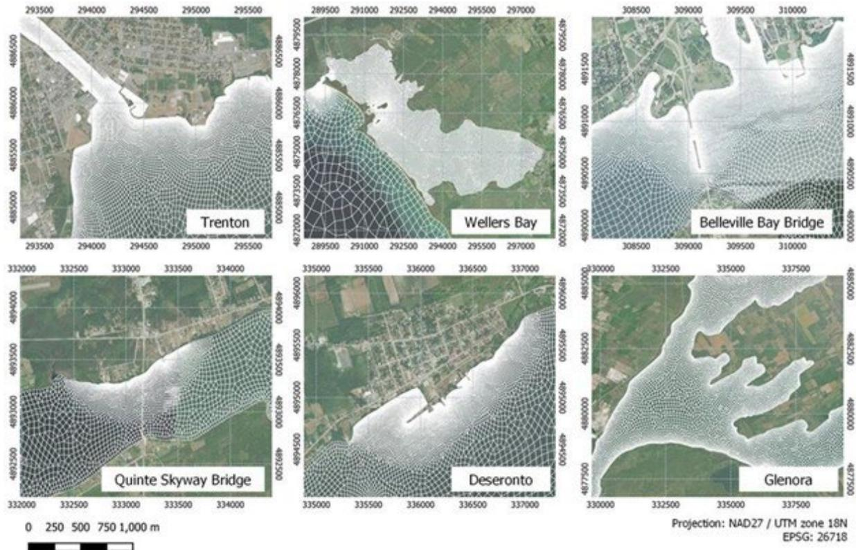
**Figure 4.12 Mesh detail at specific locations of interest within the Bay of Quinte**
