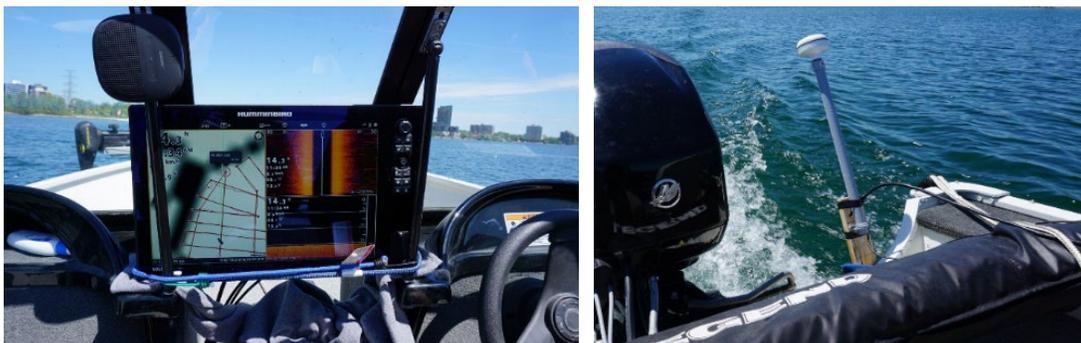
**Figure 3.15 SOLIX data collection unit and transducer mount**
