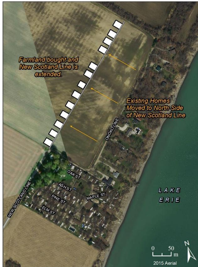
**Figure 7.5 Road and home re-alignment further inland to reduce erosion vulnerability**
