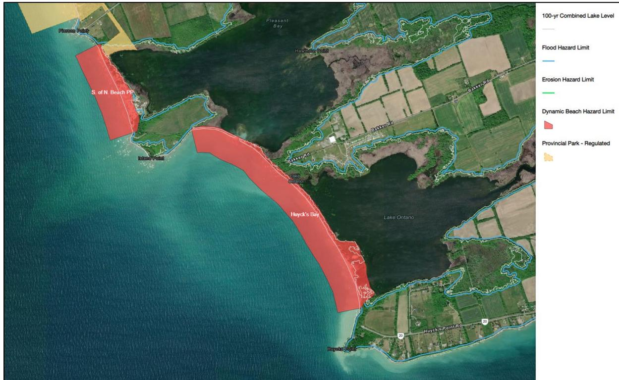
**Figure 5.8 Sample of dynamic beach hazard mapping for the southwest Prince Edward County shoreline from North Beach Provincial Park to Huyck's Point (red polygon is the dynamic beach hazard, white line is the 100-year flood level and blue line is the flooding hazard including wave uprush)**
