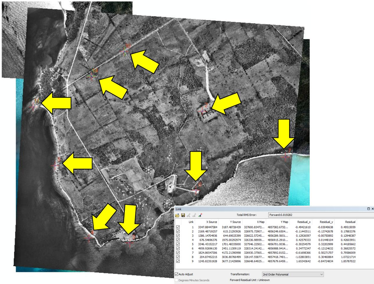
Figure 4.4 Ground control selection during photo registration
