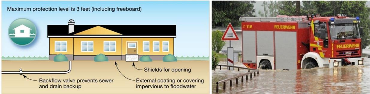
**Figure 7.3 Examples of measures for floodproofing an existing building (left) and a specialized emergency vehicle with enhanced abilities to navigate through floodwaters (right)**
