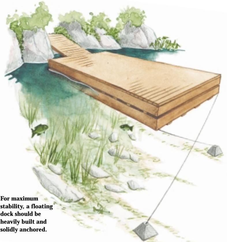
**For maximum stability, a floating dock should be heavily built and solidly anchored.**
