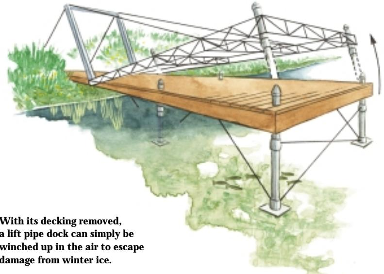
With its decking removed, a lift pipe dock can simply be winched up in the air to escape damage from winter ice.
