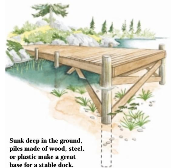
**Sunk deep in the ground, piles made of wood, steel, or plastic make a great base for a stable dock.**
