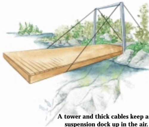
A tower and thick cables keep a suspension dock up in the air.
